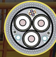
Integrated high electricity umbilical
